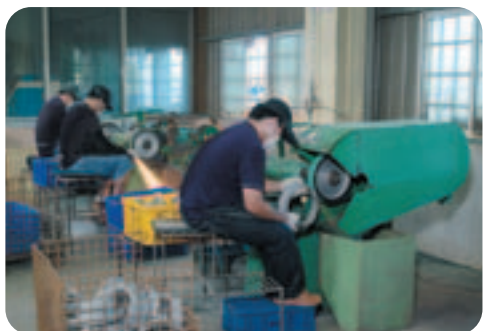
8 切割研磨 Cutting and grinding 湯口を切断・研磨
